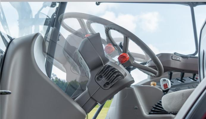
Smooth handling thanks to the steering wheel angle/height adjustment setting creates an optimal driving position, improving workability, comfort, and easy access.
