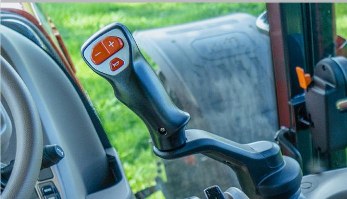
The multi-functional loader joystick is built with 3rd service and Powershift buttons, simplifying loader working conditions for the user.
