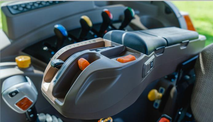
The multi-functional electronic armrest features numerous functions, such as throttle engagement, 3-point linkage lift and lower, Powershift and Auto Powershift mode.
