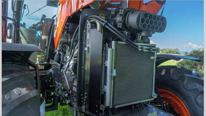
Built with a 3.8L 4 cylinder diesel engine at either 130hp or 140hp, the HX achieves optimum engine performance, thereby increasing work productivity.
