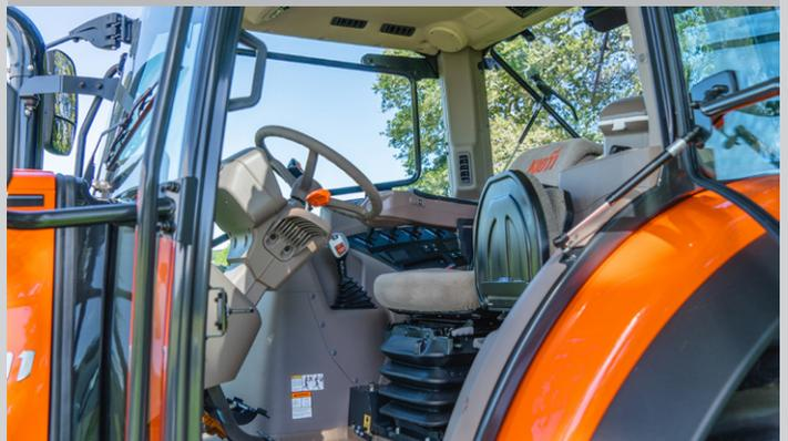
Large ergonomic cabin, with well placed instruments and features. Includes air suspension swivel seat, auxiliary seat with seatbelt, USB charging & numerous storage compartments.
