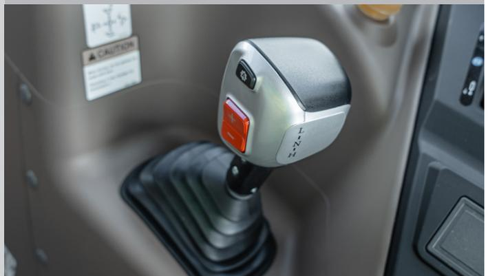
A simple button operation on the side speed lever and armrest gives you a 32x32 transmission with an 8-speed Powershift in 4 ranges.
