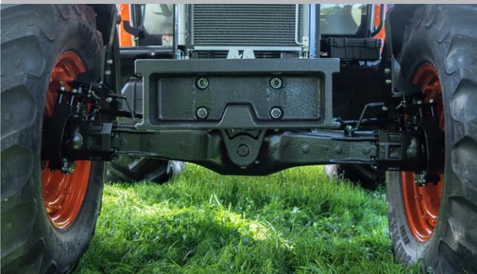
The use of a LSD front axle prevents the occurrence of slippage due to the load difference of the front wheels. This creates traction, greatly aiding manoeuvrability in any conditions.
