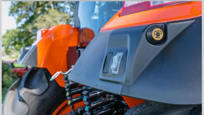
The addition of rear fender remote and PTO switches increases the convenience of both the removal and attachment of external implements.
