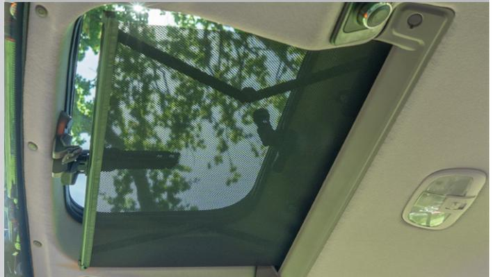
A transparent sunroof inside the cabin ensures an upward clear vision when using the loader, improving ease of operation and safety.
