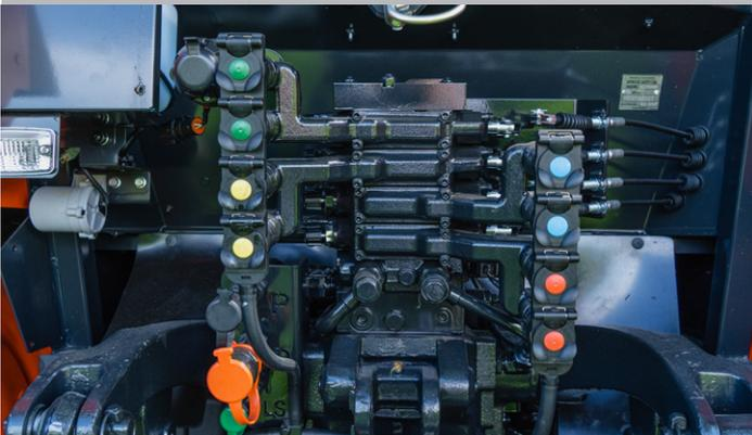
Load Sensing provides optimal hydraulic pressure and flow rate for load sensing operations. This results in automatically neutralising valves in the event of high loads during operation.
